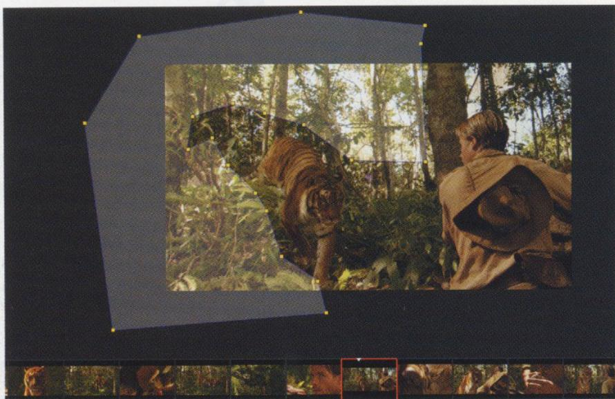
Above: The Discreet Lustre allows for "Power Windows" defined by polygons. These windows can move during the shot. The polygon shown here (also taken from the Lustre proxies) has been lightened for illustration purposes. Right: A flow chart of the hybrid DI process at Éclair, showing the different image formats used.
